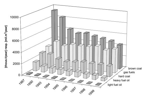
Fig. 4.5 **Development in consumption of the individual fuel types** in power industry (EAPSI 1)
