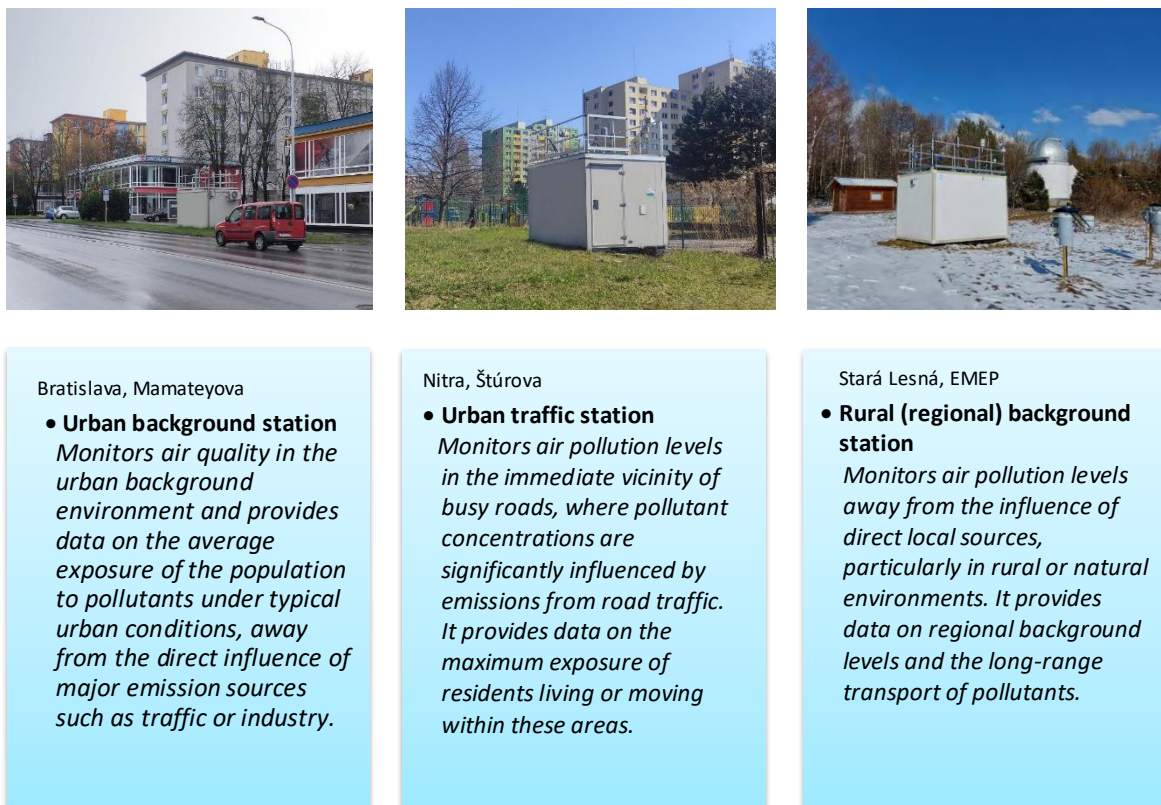
Fig. 1 Main types of automatic monitoring stations of the National Air Quality Monitoring Network.
