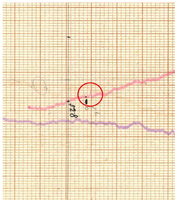
Figure 1. A section of the microbarographic record measured with the Sprung-Fuess barograph in Hurbanovo on June 30, 1908. The pressure anomaly from the Tunguska meteorite explosion is clearly noticeable at \sim 6:00 Local Mean Time (marked with a circle), i.e. at 5:47 Central European Time. One horizontal division corresponds to 10 minutes, one vertical division corresponds to air pressure of 0.1 Torr. The highlighted point value of 52.8 corresponds to the absolute pressure of 752.8 Torr.
